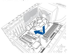
Place nine screws into the holes indicated by circles to secure the motherboard to the chassis.
